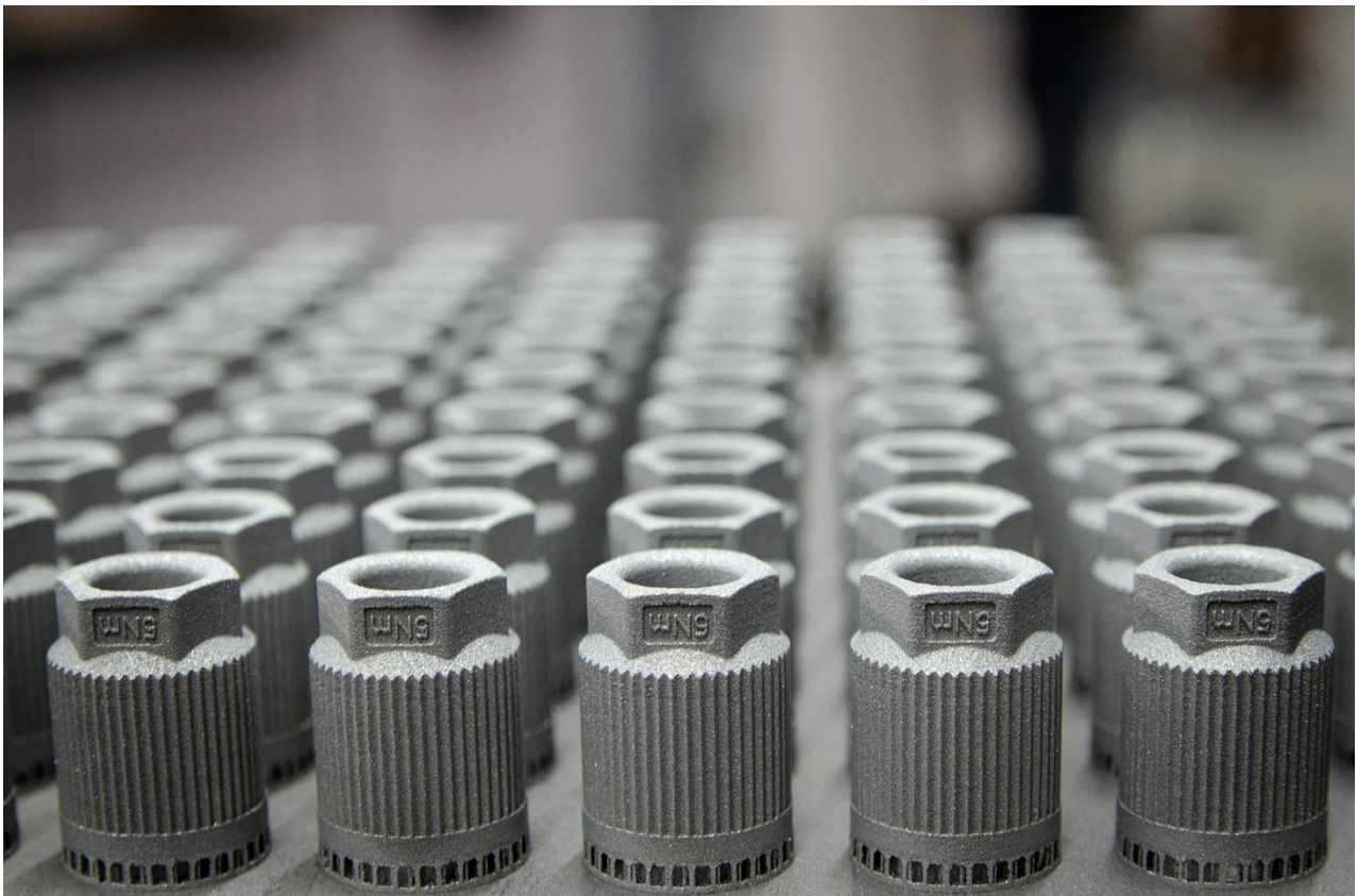
Additive manufactured small series made of Zamak 5.
