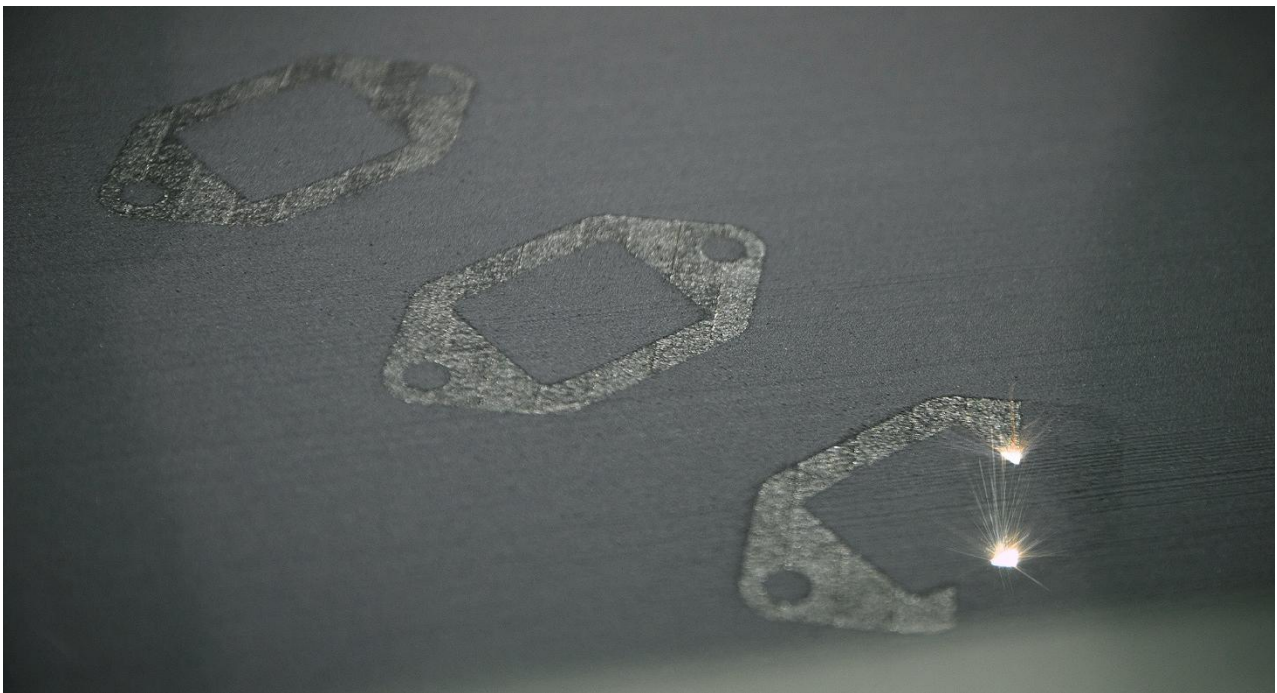
A view of the installation space during selective laser melting.
