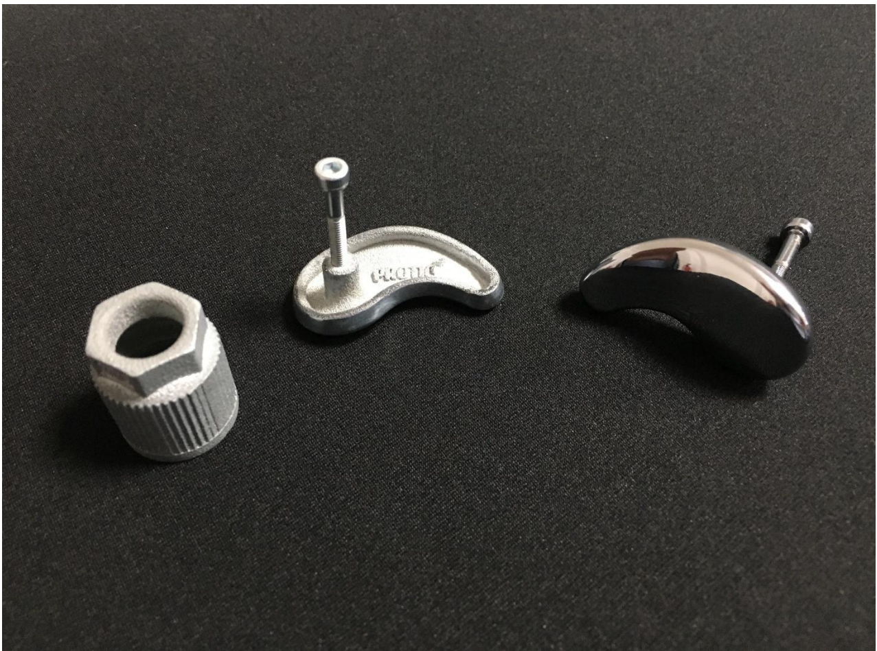
Additively manufactured components with subsequent chrome surface coating; component design and electroplating surface finishing by HDO Druckguß- und Oberflächentechnik GmbH
