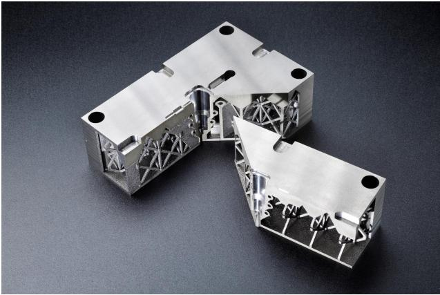
Additively manufactured injection molds with complex, near-contour cooling channels increase production performance and reduce cycle times.
