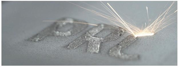
In the additive manufacturing of metal components, fine metal powder is melted together layer by layer using a powerful laser. Almost 100% of the unmelted powder can be reused after the process.
