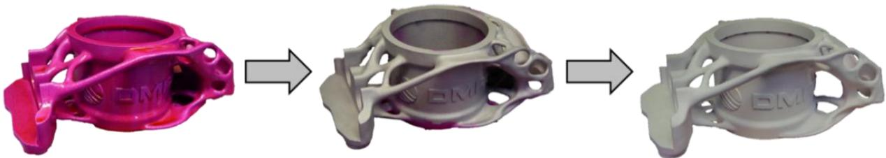
**Graphic 3:** Dye penetration test according to ISO 3452 using the example of a wheel carrier
