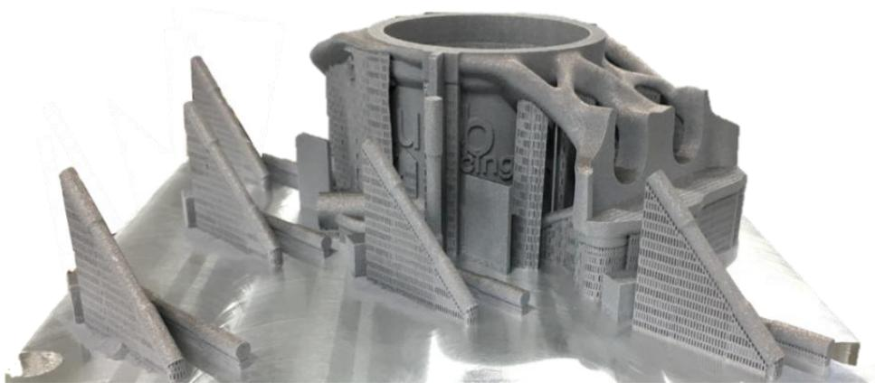
**Graphic 2:** Validation of the quality assurance concept using a laser-melted wheel carrier from the Direct Manufacturing Research Center at Paderborn University
