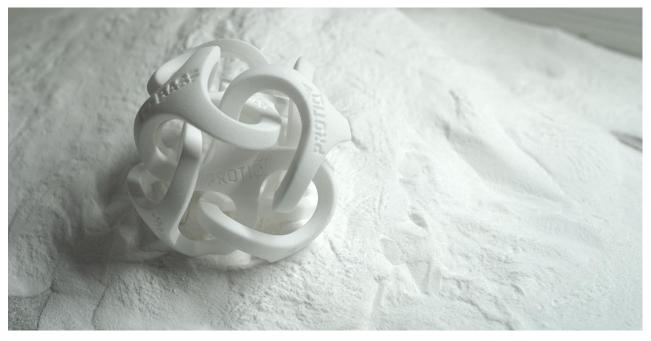
The SLS process enables the production of highly complex components and offers great design freedom during development.
