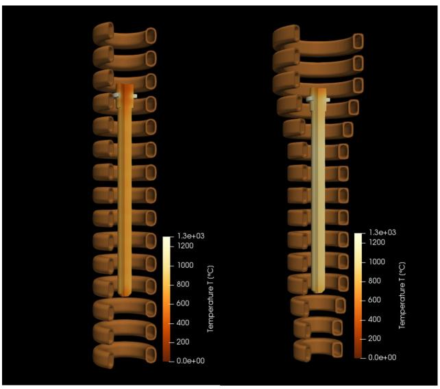
The coils optimized by simulation allow for more precise heating and reduced cycle times (left a conventional coil geometry, right the optimized coil with improved heating behavior)
