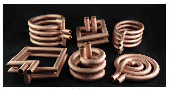
The process developed by Protiq for processing highly conductive pure copper in a selective laser melting process enables the production of innovative components for the electrical industry
