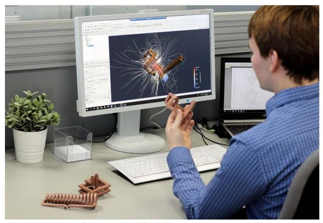
The additive manufacturing of induction coils made from highly conductive copper materials offers new possibilities for producing even more complex coil geometries; the optimized inductors are determined at Protiq using numerical simulation methods
