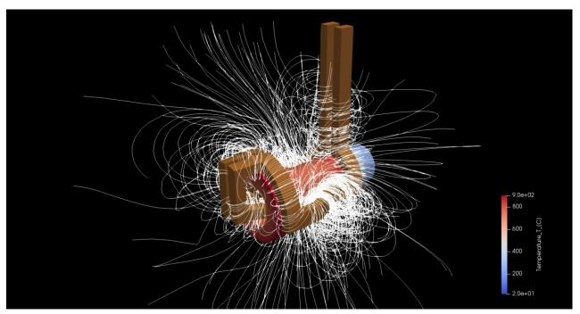
The numerical simulation of the inductive heating process can avoid expensive tests; the simulation results enable a detailed analysis of the electromagnetic behavior
