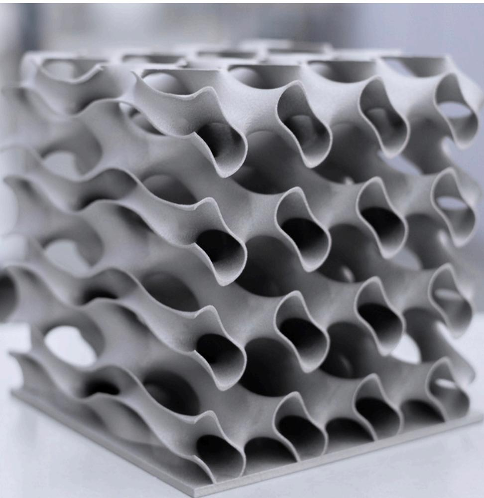
**The production of prototypes from zinc previously required a lot of time and money. However, this problem can now be solved with the help of additive manufacturing: A process developed by PROTIQ allows components to be produced from Zamak 5 using 3D printing.**
