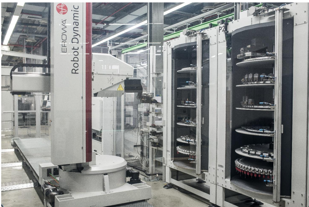
Fully interlinked, automated production cell in the internal tool shop of Phoenix Contact GmbH & Co. KG as an example of the consistent implementation of Industry 4.0.
