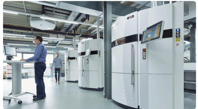
Thanks to automated powder handling, the systems in plastic laser sintering are continuously supplied with build powder
